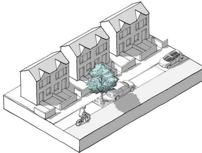
A street tree integrated between on-street parking.(Credit: NMDC)
